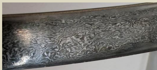
Patterns on Damascene style steel (candlepowerforums.ru)
